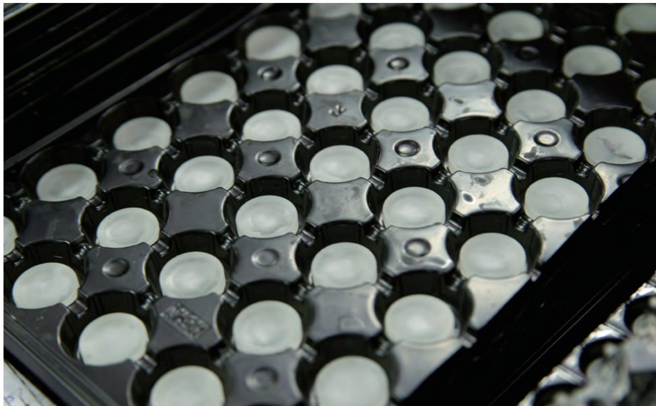
Glass used for relatively small lenses. The degree of transparency remains poor at this stage.
