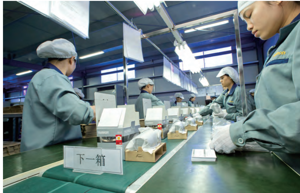
Packaging is carried out on assembly lines. The number of packages to be packed each day is set according to timing and by type of lens.
