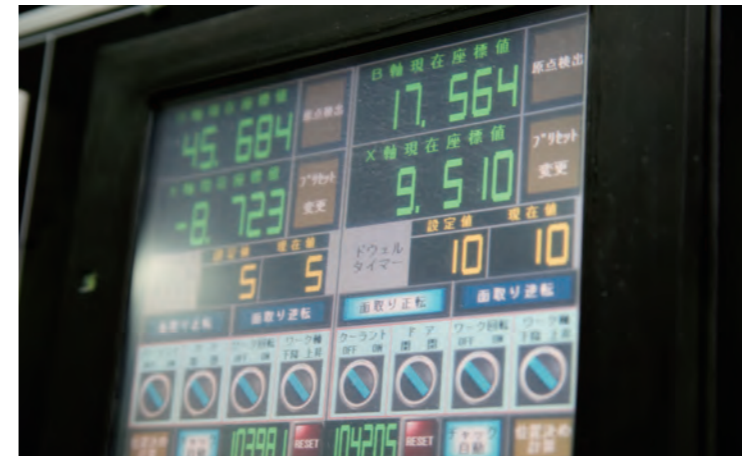
The monitor shows the rotation speed, thickness and angles of the grinding machine.
