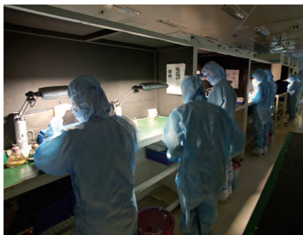
The point at which the outer appearance is checked and where the lenses are adhered to each other are in the same operations line.
