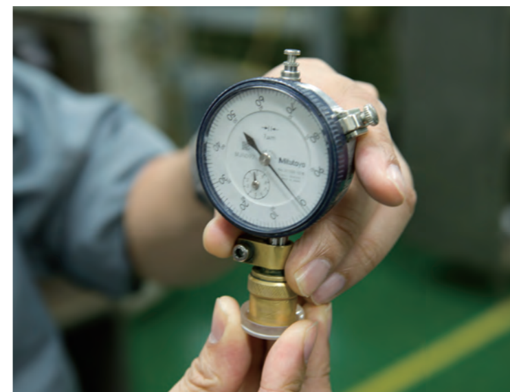
This tool measures the R of the roughly scraped lenses. If the gauge reads “0,” it means the rough grinding has been completed and the lens continues to the next process.
