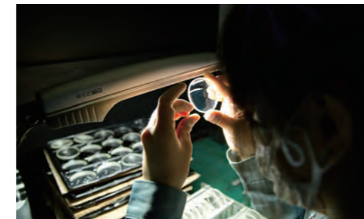
Appearance precision inspection: A visual examination is carried out to identify any flaws or dirt by casting light on the lens. If a defect is found, the lens is returned to be ground once more.
