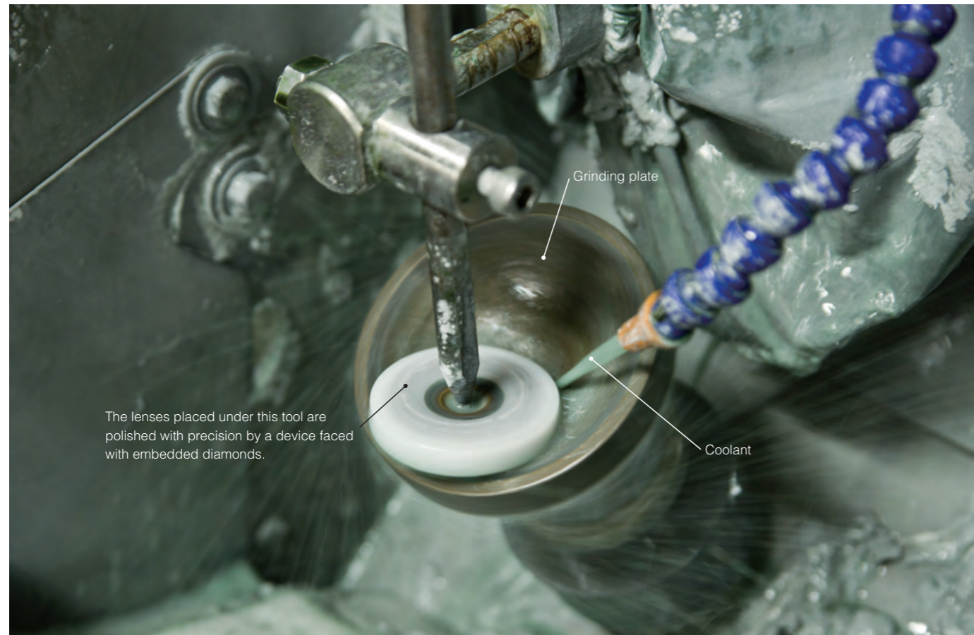
Precision grinding. During the process, a coolant is used to reduce friction heat created between the lens and the diamond pellets.
