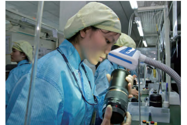
A visual check is then conducted for overall operation, the exterior, debris or marks – concluding the Main-line assembly process for the lens unit.
