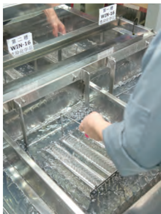
The time spent on cleaning lenses is different in each of the tanks. After a specific period, the lenses are transferred from one tank to the next.
