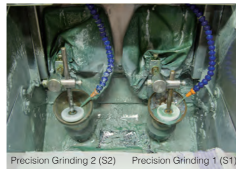
The process has two steps, “Precision Grinding 1” (S1) and “Precision Grinding 2” (S2), which are conducted in adjacent parts of the machine.
