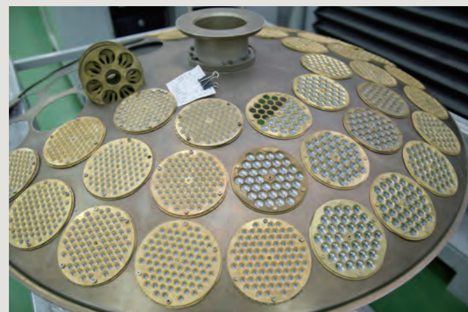
The coating dome. Before being coated, lenses are placed in an umbrella-like dome and installed on the upper right section of the device, as seen on p.19. This picture shows a coating dome for relatively small lenses.
