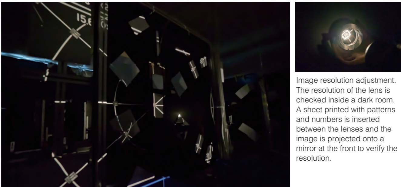
There are specific scales and standards to test the visibility of the numbers and patterns that are projected onto the mirrors.
