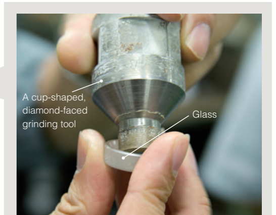
The process to shape the glass into a concave lens. The cup-shaped, diamond-faced tool rotates to roughly grind the glass.
