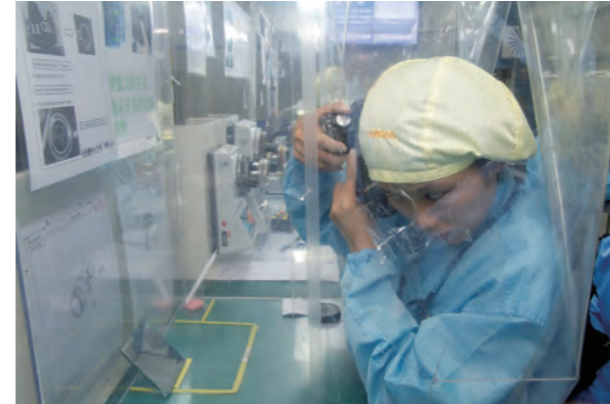
The lens is attached to the camera and a technician checks the AF/MF switch, the level of operating noise and overall smooth operation.
