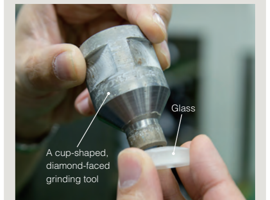
The process to shape the glass into a convex lens.
