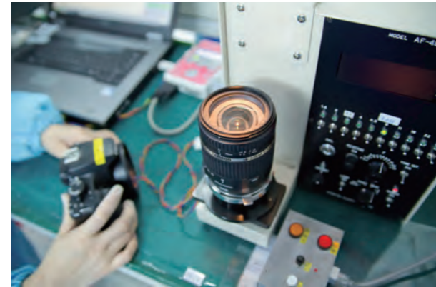
The camera and lens are connected by a cord to check the precision of the diaphragm as well as aperture diameters.
