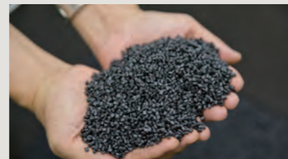
Plastic pellets that are used to make the components. The ratio at which the plastics are combined is altered for each component.
