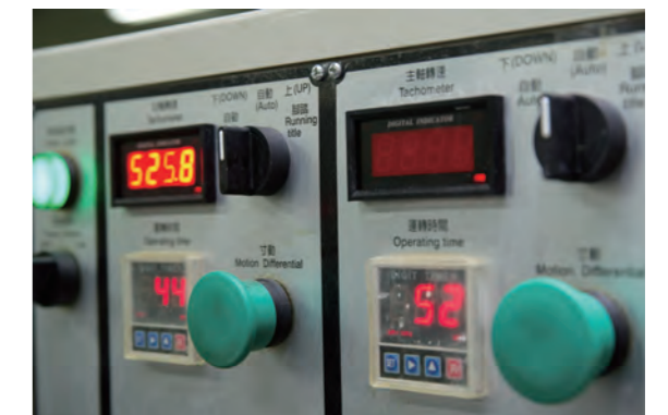
The machine operator sets the speed and duration of the rotation for precision grinding.
