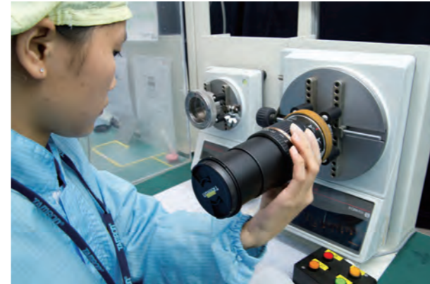
A technician rotates the zoom lens to get a feel for the torque and response.
