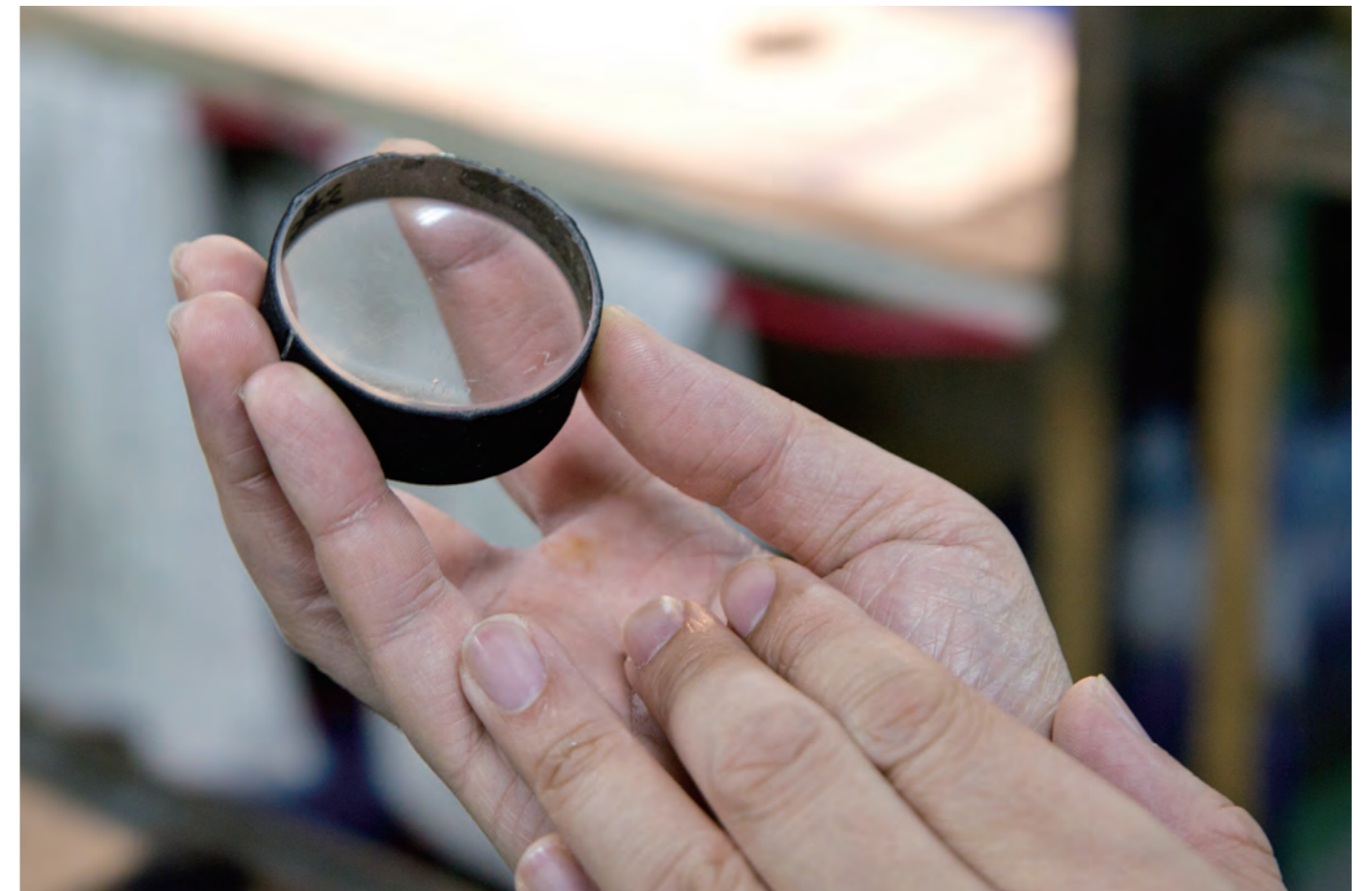
A test plate. A test plate is a sample that represents the desired shape of the lens, with lenses required to conform to the test plate. The accuracy of R is measured using this test plate.
