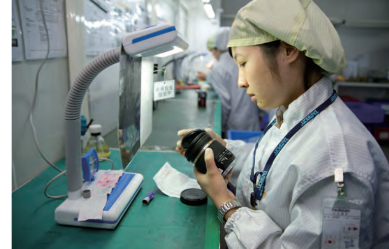
The product is then taken to the quality assurance department for a final check. Here, a fresh pair of eyes will give the unit a final once-over, check the exterior and test the camera.
