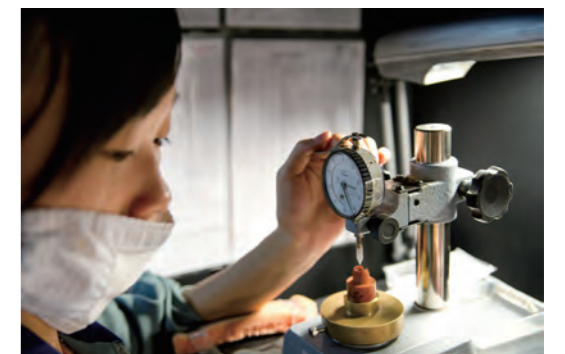
Core thickness inspection: A precision instrument is used to examine the thickness.
