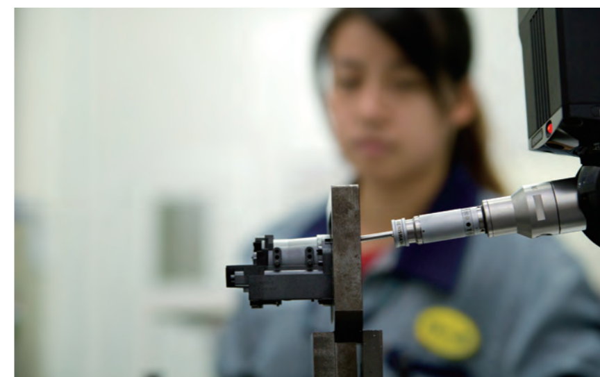
The finished components are taken to a different room for the form and groove widths to be inspected. A three-dimensional measuring device with precision down to 1 micron is used to check the accuracy.
